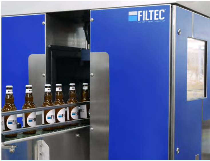
FILTEC Vision Enclosure Inspects Glue-on Labels on Bottles
