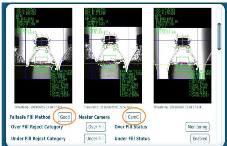
Each fill level inspection camera is run independently. Images are combined to compensate for product slosh and provide accurate fill level measurement.
